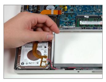
Lift the hard drive retaining bracket up and out of the computer.
